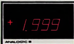
stroom DC 4-20 mA of 10-50 mA
